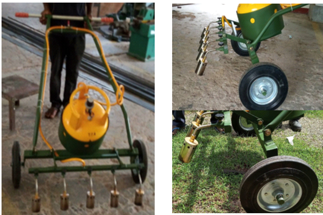
Figure 1b. Flame weeder – Front elevation (Left); Burner alignment and gas supply (top right); Burner mount and gas regulation (bottom right)
