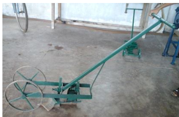
Figure 2. Assembled view of developed mould board weeder
